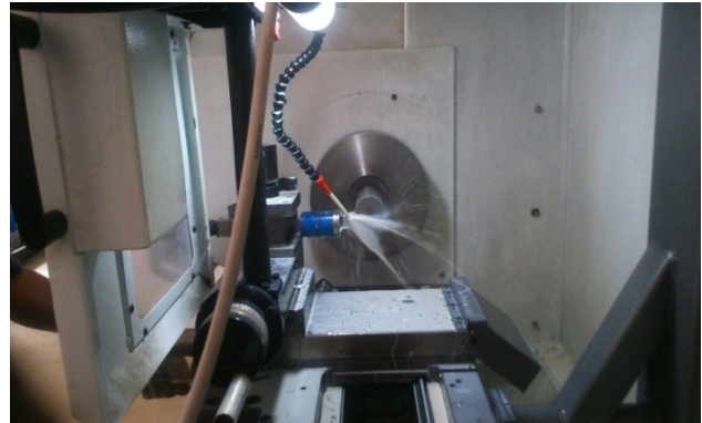
Figure 5: Machining under flooded condition
