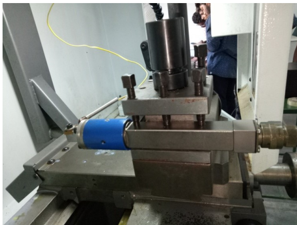
Figure 8: Tool-work interface thermocouple insulated and coupled with the tool holder
